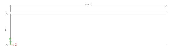
In the middle of the bridge deck an internal edge is created. Using the **Cursor Snap Settings** you can snap on midpoints of the long edges so the edge can be imported through the option
